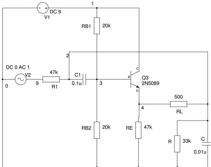
Figure 9: Same voltage divider implemented using the BJT gyrator
