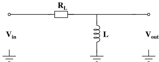
Figure 6: Inductor with internal resistance  $R_L$  and inductance  $L$
