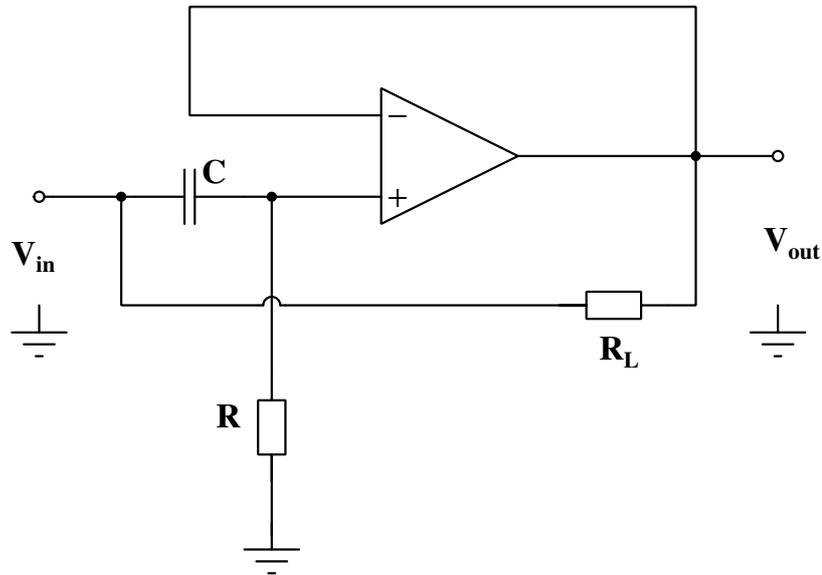
Figure 5: Gyrator using a BJT, inductance  $L = R_L RC$ .
