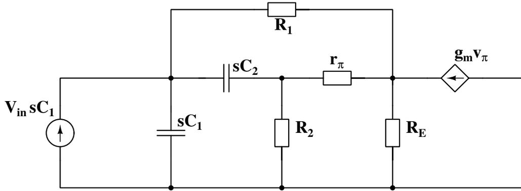
Figure 3: Small-signal model of the BJT high-pass filter
