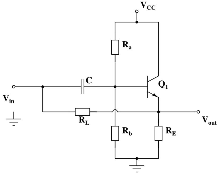
Figure 7: Gyrator using a BJT, inductance  $L = R_L(R_a || R_b)C$ .
