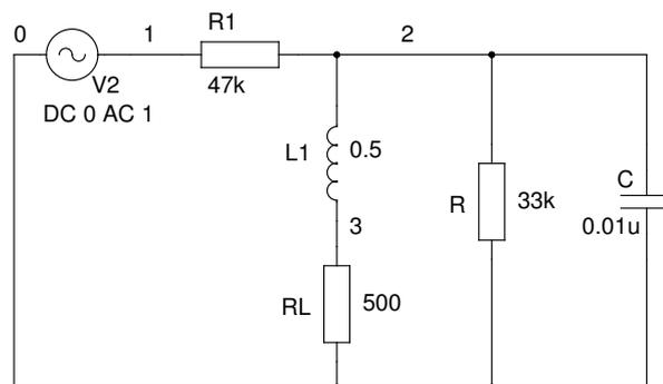
Figure 8: Schematic of a voltage divider using a RLC resonance circuit
