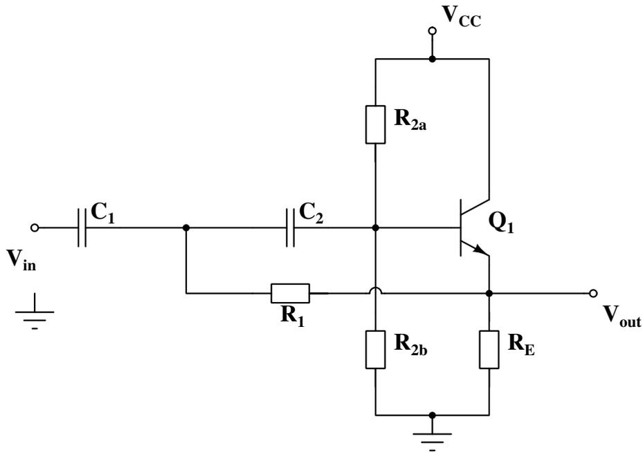
Figure 2: A high-pass Sallen and Key filter using a BJT emitter follower
