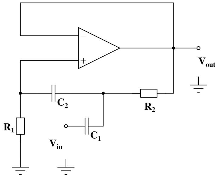
Figure 1: A high-pass Sallen and Key filter using an op-amp
